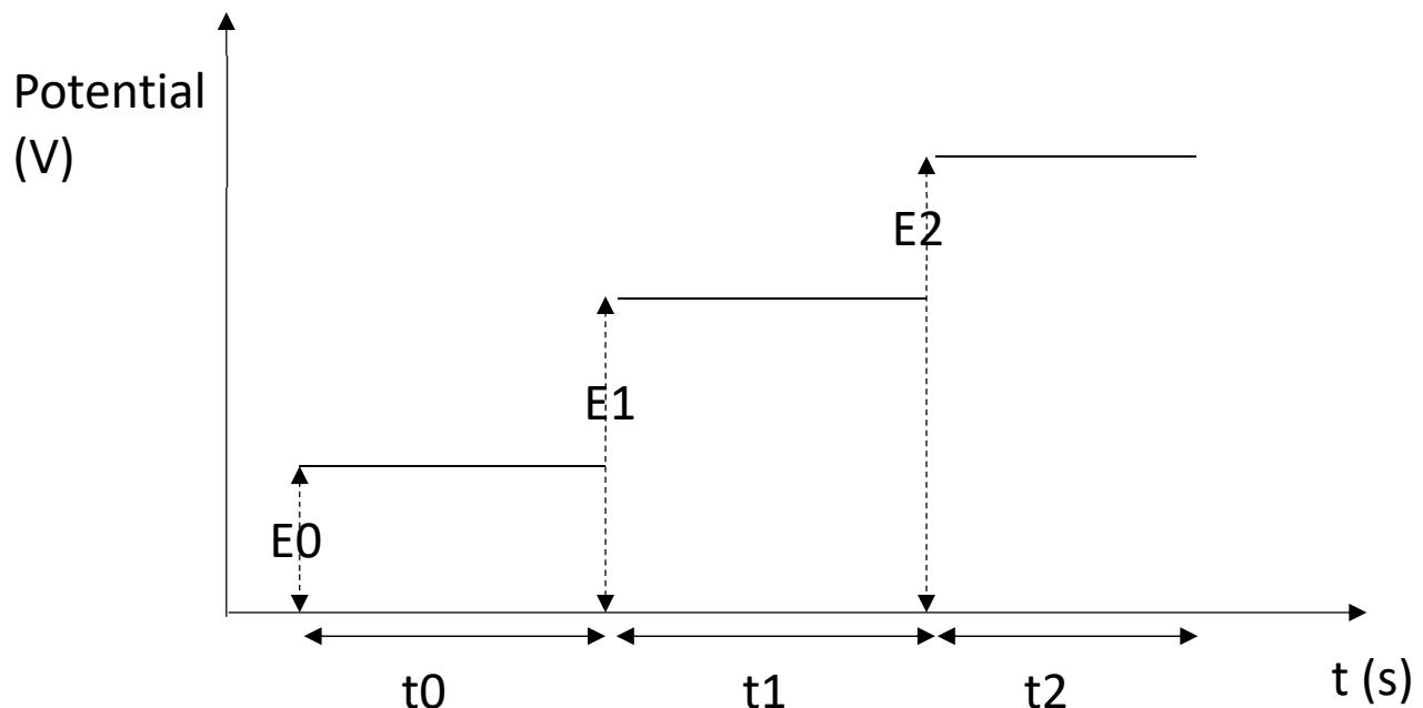
Figure 2 potential excitation wave in Chronoamperometry. E0: initial potential; E1: potential step 1; E2: potential step 2; t0: initial time; t1: potential step 1 time; t2: potential step 2 time.
