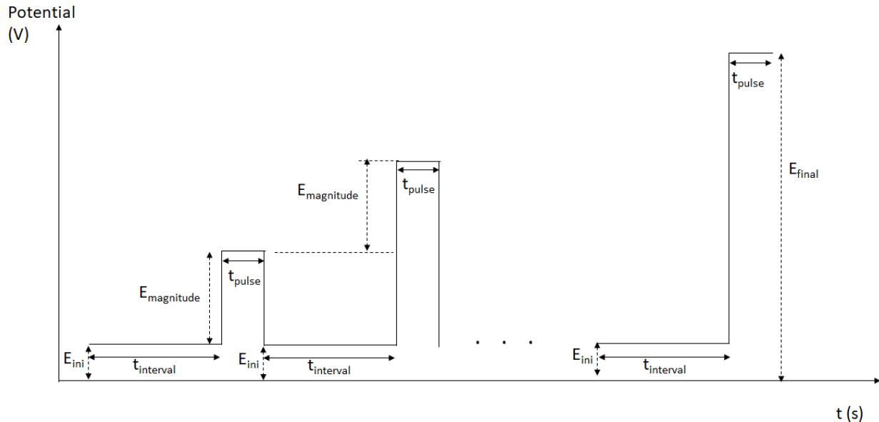
Figure 4 potential excitation wave in Normal Pulse Voltammetry.  $E_{ini}$ : initial E;  $E_{final}$ : final E;  $E_{magnitude}$ : pulse magnitude;  $t_{interval}$ : pulse interval;  $t_{pulse}$ : pulse width;
