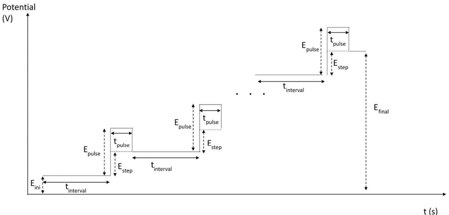
Figure 3 potential excitation wave in Differential Pulse Voltammetry.  $E_{ini}$ : initial E;  $E_{final}$ : final E;  $E_{step}$ : step E;  $E_{pulse}$ : pulse height;  $t_{interval}$ : pulse interval;  $t_{pulse}$ : pulse width;
