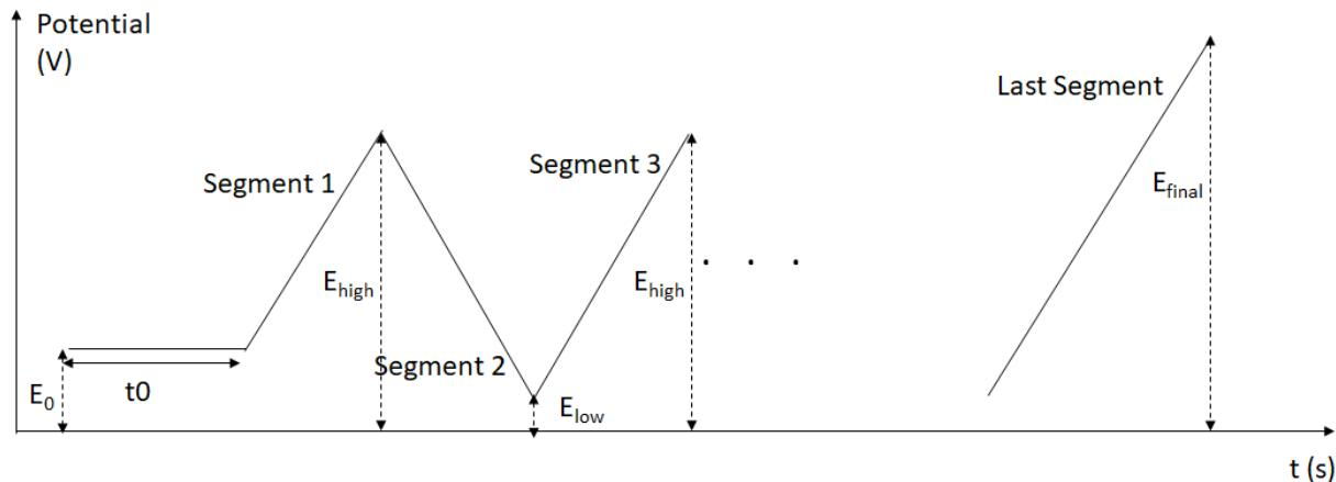
Figure 1 potential excitation wave in Cyclic Voltammetry.  $E_0$ : initial potential;  $t_0$ : waiting time;  $E_{\text{high}}$ : high potential;  $E_{\text{low}}$ : low potential;  $E_{\text{final}}$ : final potential;
