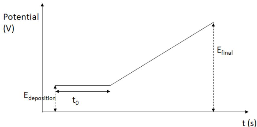
Figure 6 potential excitation wave in Stripping Linear Scan Voltammetry.  $E_{\text{deposition}}$ : deposition potential;  $E_{\text{final}}$ : final potential;  $t_0$ : deposition time
