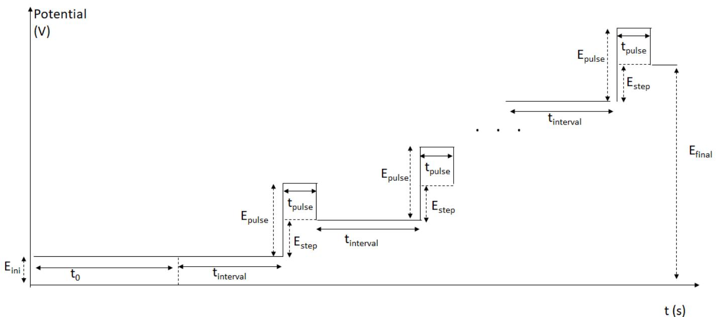
Figure 5 potential excitation wave in Stripping Differential Pulse Voltammetry.  $E_{ini}$ : deposition potential;  $E_{final}$ : final potential;  $E_{step}$ : step E;  $E_{pulse}$ : pulse height;  $t_{interval}$ : pulse interval;  $t_{pulse}$ : pulse width;  $t_0$ : deposition time
